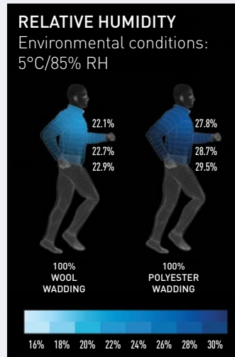
Figure 2: Wool-filled jackets keep the skin microclimate drier (left) and warmer (right) across the torso, compared to polyester-filled jackets. This has been tested in cold, damp conditions during walking at 5°Celsius/85% relative humidity.
